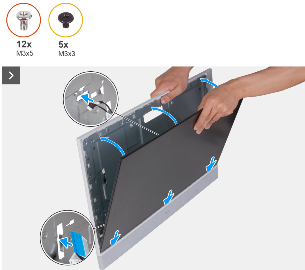
Figure 65. Installing the display panel
