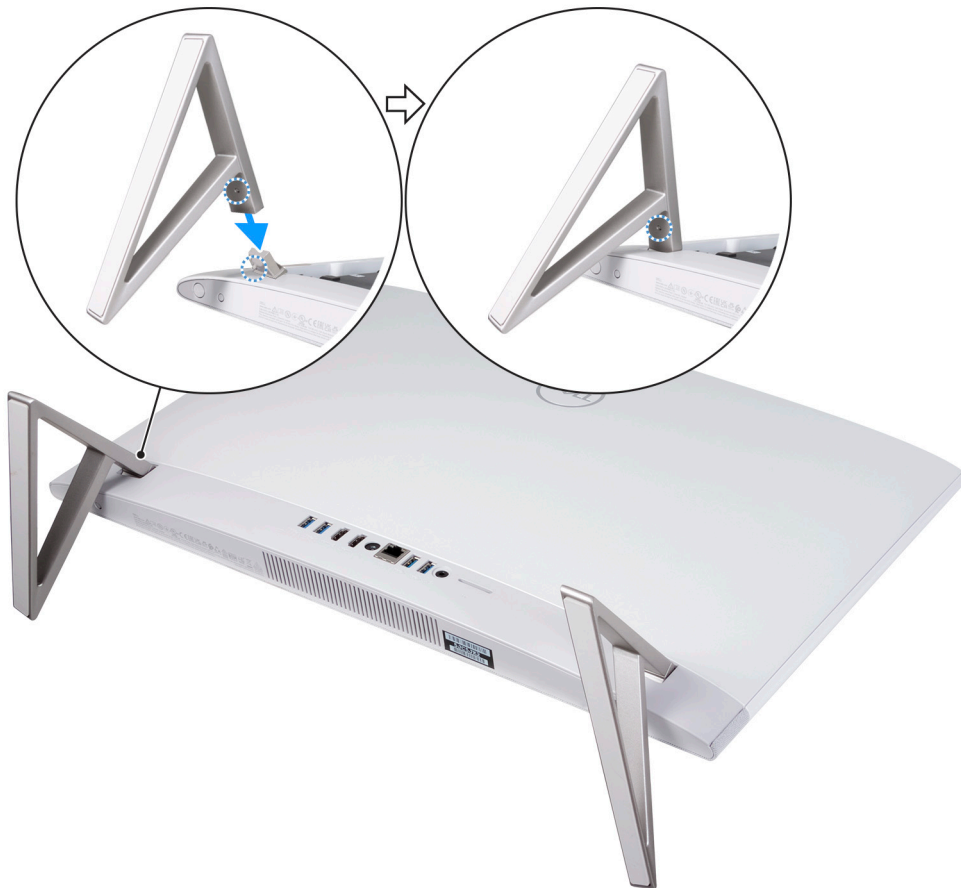
Figure 8. Installing the stand
